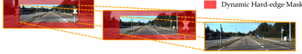
Fig. 3. The sketch of dynamic hard-edge mask (the red part). For better display, the frame-to-frame time between these 3 frames is \sim 0.5s , so the mask is much larger than actual mask we used in experiments.
