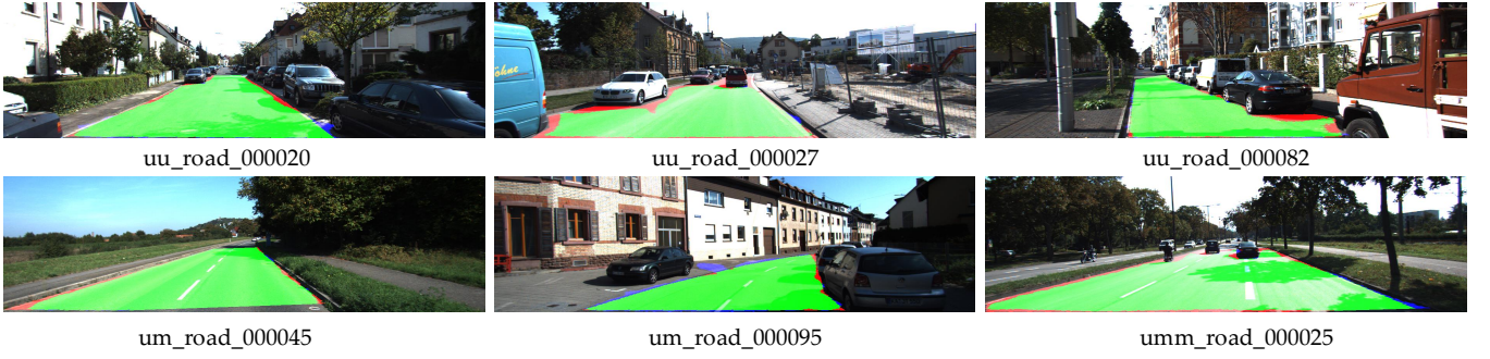
Fig. 6. Exemplar results on the KITTI server. The green, blue and red regions denote respectively true positives, false positives and false negatives.
