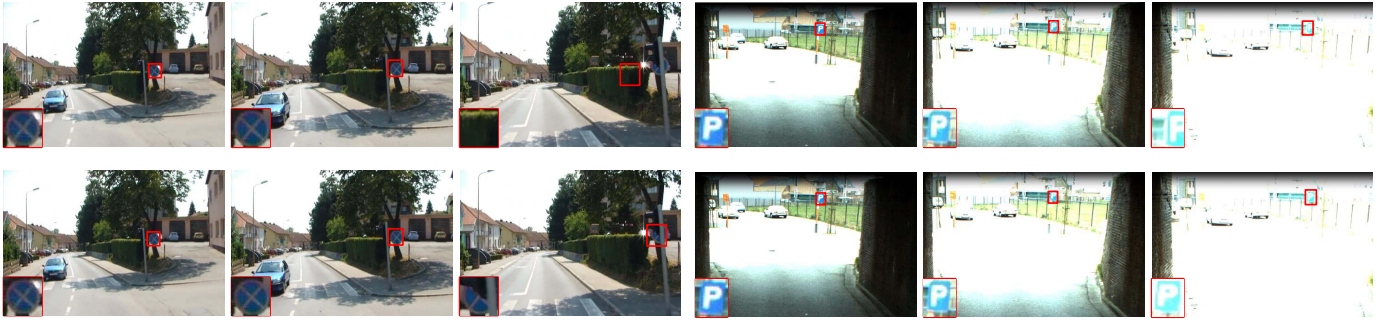
Fig. 12. The first row is the tracking only with KF, while the second shows the results of tracking with KF and on-line detection.
