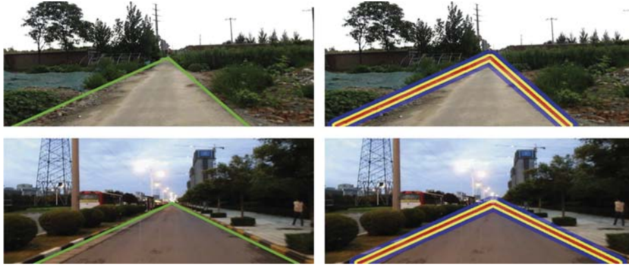
Fig. 3. Illustration of training sample selection. For the left images, the green lines indicate the ground truth road boundary. For the right images, positive instances can be randomly selected from the red region and negative ones from the blue region. The yellow region is served as a transition area. (For interpretation of the references to color in this figure caption, the reader is referred to the web version of this paper.)
